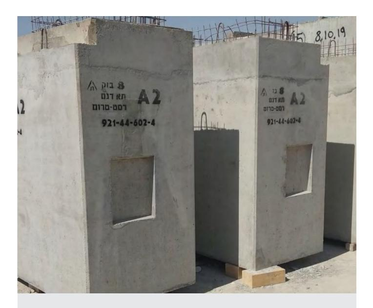
The Company's capabilities, as a leading company in the industry of precast elements and infrastructures in Israel, include manufacture of various infrastructure products, including Bezeq and multi-tubular chambers, conduits, water culverts, precast ducts, pillars, cornices, foundations for lighting poles etc.
