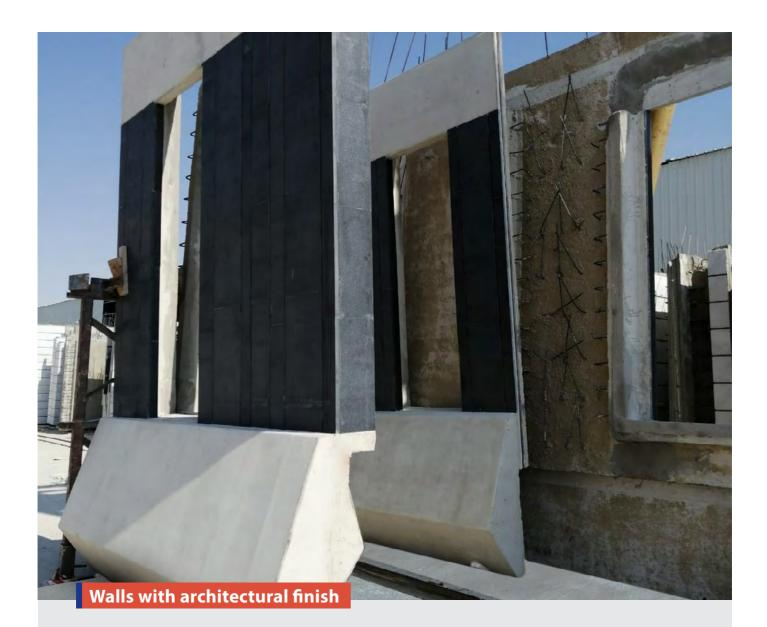
Ramet Trom manufactures walls with architectural finish using customized forms, including smooth forms to achieve special textured finishes and others. The Company manufactures precast walls with architectural finish for a wide variety of projects.
